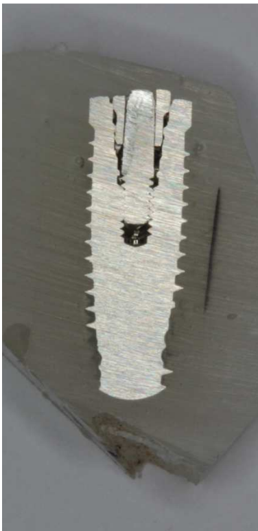
Figure 27: Fractured titanium specimen.
