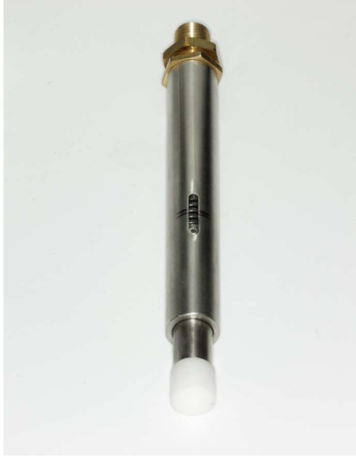
Figure 14: Loading piston for fatigue stimulation device.
