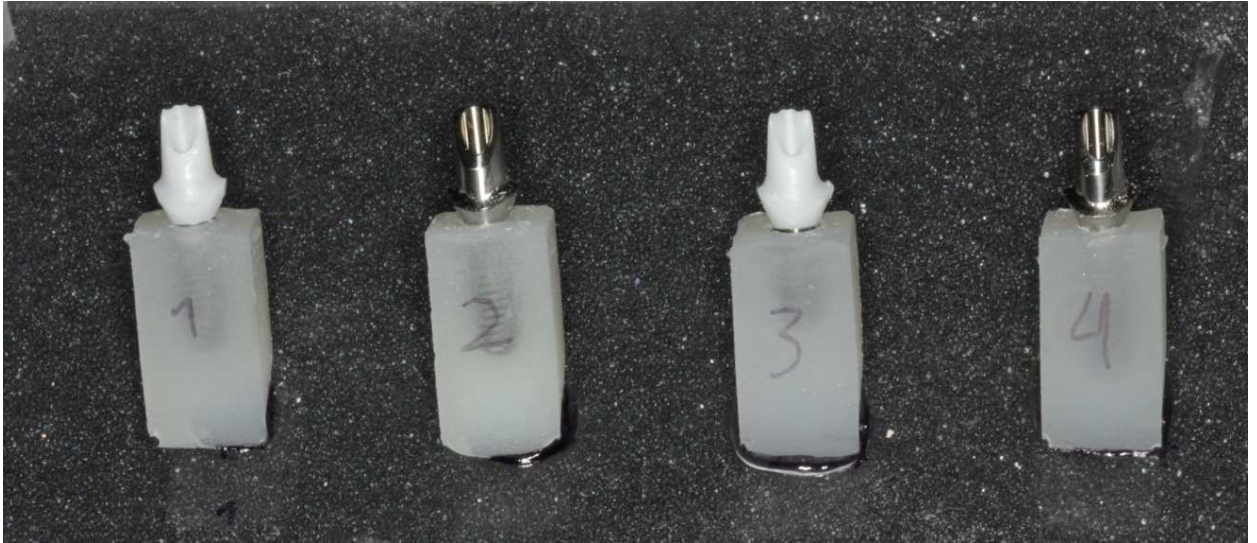
Figure 15: Mounted titanium and modified zirconia abutments at 30 degree angulation.
