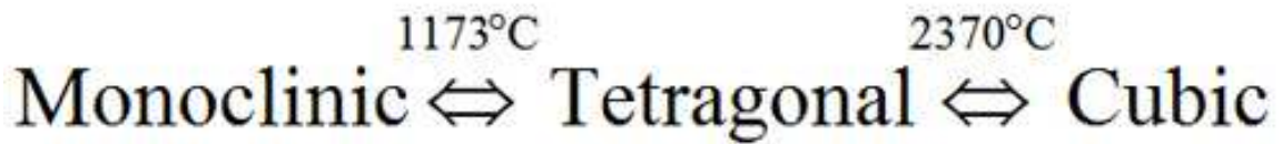
Figure 3: Ranges of Stability for the Crystallographic Phases of Zirconia
