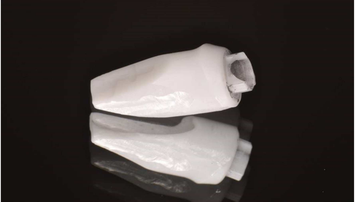
Figure 37: Fractured zirconia abutment.
