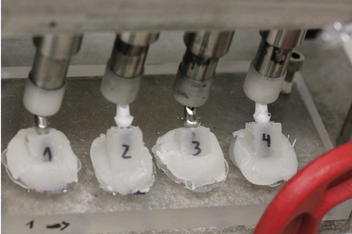
Figure 19: Specimens mounted and secured at the testing device during loading. Titanium specimens #1,3, Zirconia specimens #2,4.
