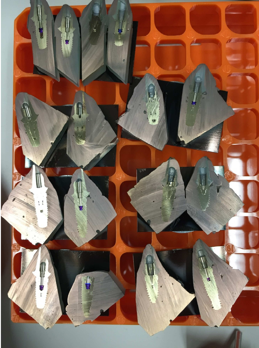
Figure 24: Specimens coated with gold for SEM imaging.
